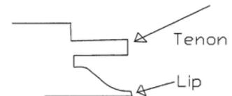
7. The rails are cut with the material face down. When cut properly the profile should produce a female cut in the end of the material with a profile and a tenon. There should be an approximately 3/64 to 1/16" lip between the profile and the face of the material. Adjust as necessary to produce this lip.
